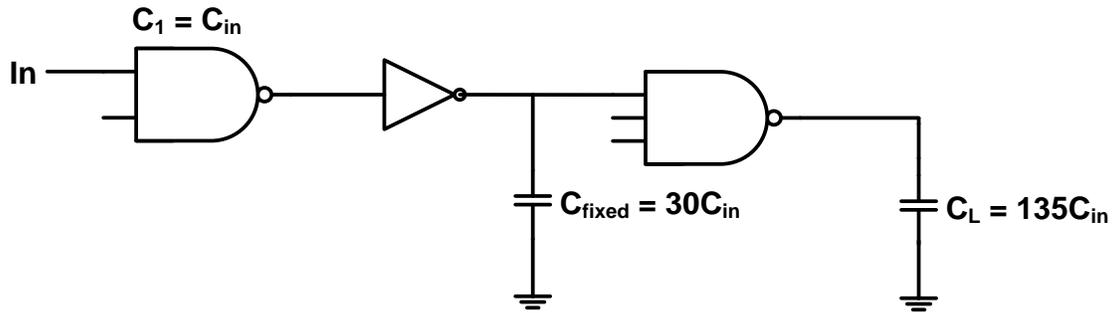
Consider the logic chain shown above, where  $C_{in} = 1\text{fF}$ . There is a fixed (i.e., independent of sizing) capacitance of  $C_{fixed} = 30C_{in}$  between the inverter and the final NAND3 gate. This fixed capacitance is sometimes called a side-load.
