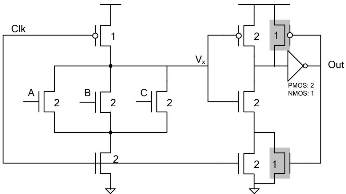
The circuit above (with relative transistor sizes annotated) is a Limited Switch Dynamic Logic (LSDL) NOR3 gate, which is essentially a dynamic gate followed by a latch.
