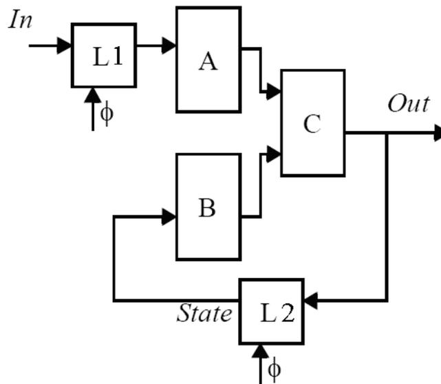
Consider the simple state machine shown above. A, B, and C represent combinational logic blocks with the following properties:
