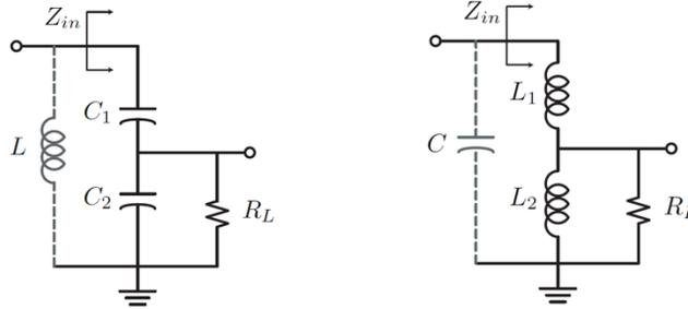
$$v_o = v_{C_2} = jX_2 \times i = v_i \frac{X_2}{X_1 + X_2} = v_i \frac{1}{1 + \frac{C_2}{C_1}} = kv_i$$
