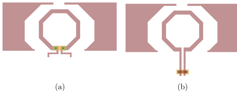
Figure 7.14: (a) An LC tank layout employing a ring inductor and two series connected MIM capacitors. (b) An inferior LC tank layout due to extra lead inductance and loss.
